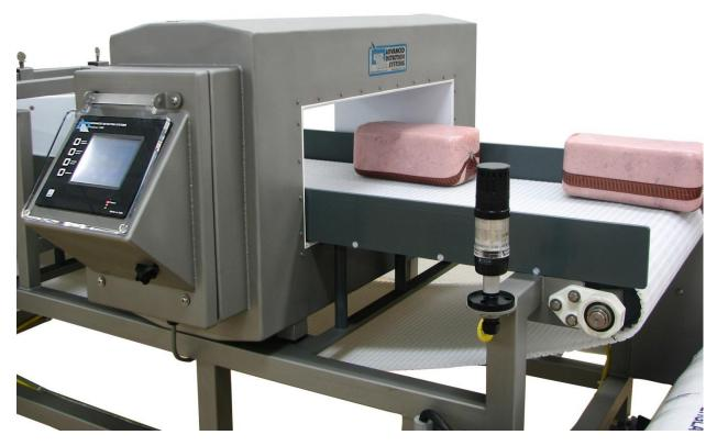
**Product Effect** is a term used to quantify the magnetic and conductive fingerprint of a product for metal detection purposes. All products have a product effect, and metal detectors must factor the magnetic and conductive properties of the product and the environment into the mathematical equation of determining detector sensitivity and detection capability.
