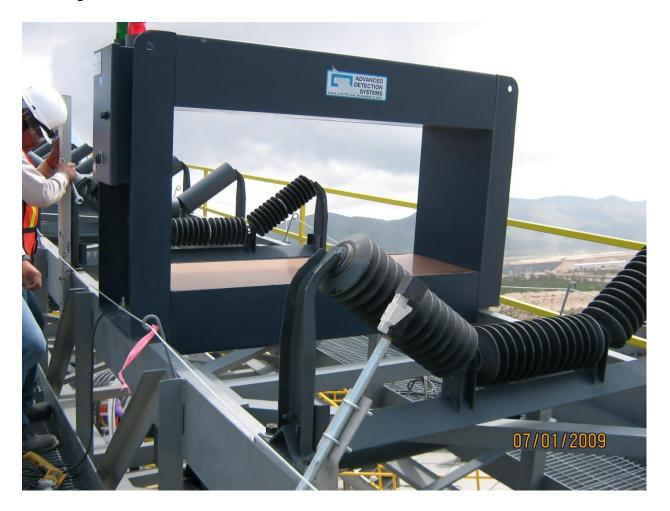
With that in mind, the Protector HD is built specifically to standard belt widths, and the aperture of the detector is always 6 inches greater than the belt width. This provides 3 inches of space on each side of the belt to prevent unwanted contact with the detector.
