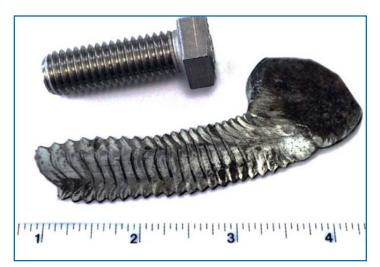
This is what's left of a 3-inch steel bolt that made its way through a roller mill. Unfortunately, the customer didn't use metal detection until after this bolt damaged the mill and caused thousands of dollars in damage. After repairs, loss of production time, and man hours to repair the equipment, the damages from this incident exceeded the cost of a new metal detector!
