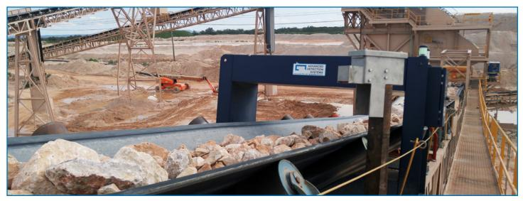
a common sight at any mineral processing facility; over-the-belt fixed magnets removing tramp metal from the product stream and protecting downstream crushers. With growing production demands placed on staff and equipment, and with a growing trend of utilizing recycled materials, the magnet-only operation is at risk.
