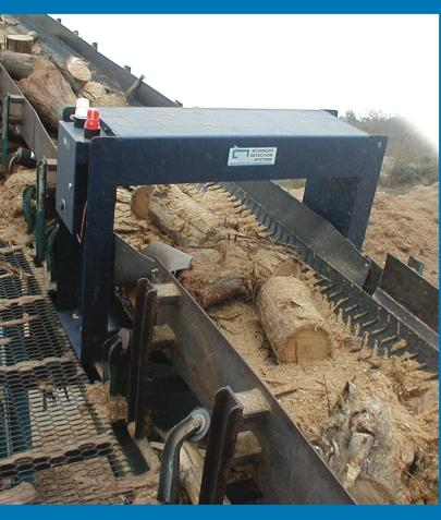
Upstream Feeding Equipment Armed with Metal Detection will Defend Your Processing Equipment and Ensure Product Purity.
