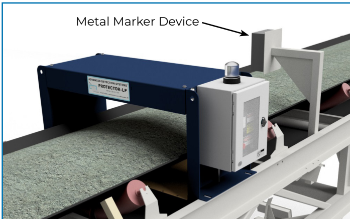
Metal Marker Device Installed on Troughed Belt
