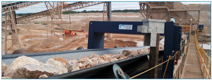
a common sight at any mineral processing facility; over-the-belt fixed magnets removing tramp metal from the product stream and protecting downstream crushers. With growing production demands placed on staff and equipment, and with a growing trend of utilizing recycled materials, the magnet-only operation is at risk.
