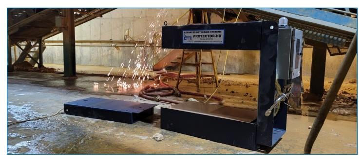
polymer idlers is recommended. Safety rails or other overburden devices must be replaced with nonmagnetic materials such as wood, PVC or fiberglass. Any metal within the metal-free zone will upset the balance of the field and compromise the detection levels of the unit.
