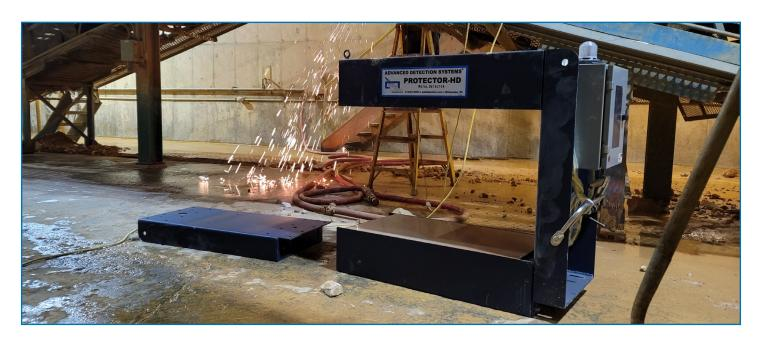
on either side of the detector. If idlers cannot be removed, then replacement with non-magnetic polymer idlers is recommended. Safety rails or other overburden devices must be replaced with non-magnetic materials such as wood, PVC or fiberglass. Any metal within the metal-free zone will upset the balance of the field and compromise the detection levels of the unit.
